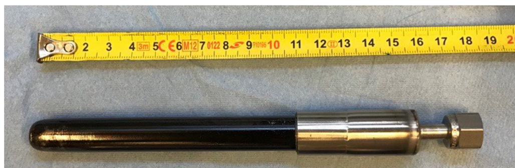
Figure 2. Double-skinned membrane with a fingerlike configuration and the other end sealed.
