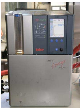
Figure 2.3.1 Thermo regulator Huber-Unistat Tango Nuevo for accurate temperature regulation
