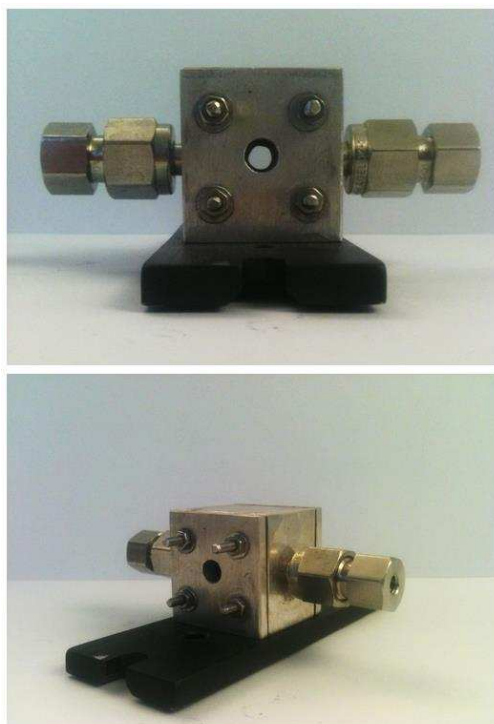
Figure 2.2.4 High pressure UV cell for liquid ammonia studies
