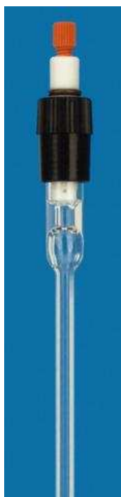
Figure 2.2.3 Diagram of high pressure NMR tube.
