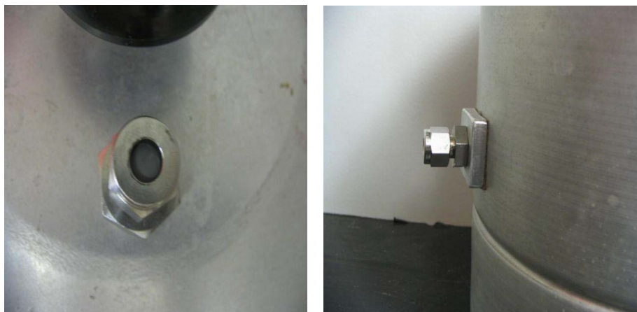
Figure 3.5 A photograph of bulkhead septum valves. On the left is the top inlet valve and right is the bottom outlet valve.
