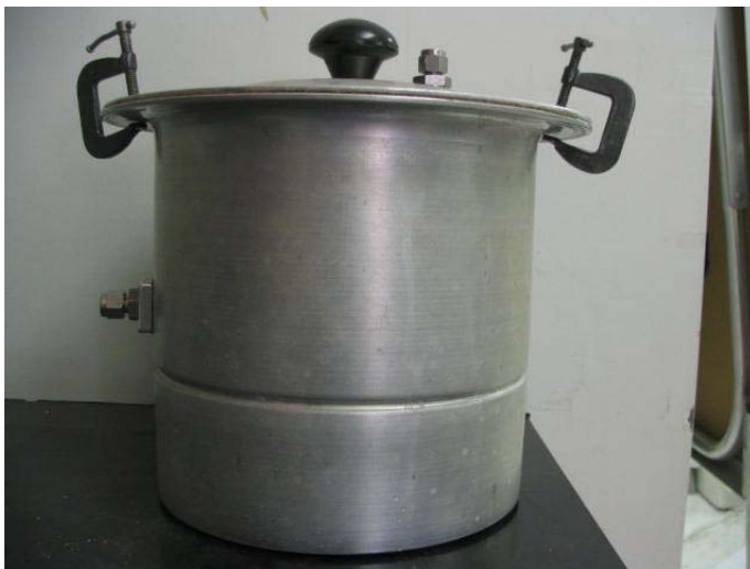
Figure 3.4 A photograph of aluminum desiccator with two bulkheads with air tight septum.
