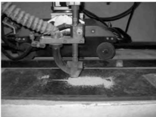
Fig. 1 - Submerged Arc Welding equipment used in the fabrication
