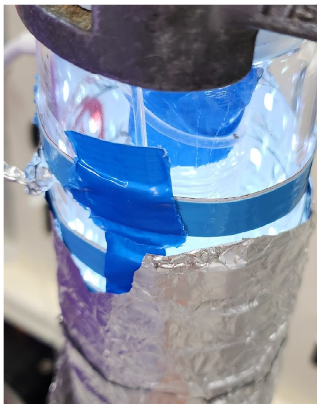
Figure 19: The flow photoreactor, showing inner flow tubing and the LED strip secured on the outside.
