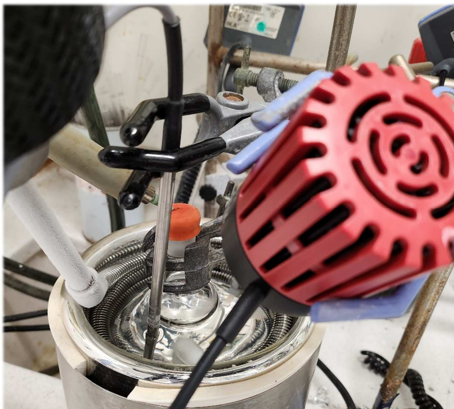
Figure 17: The setup for photochemical irradiation.
