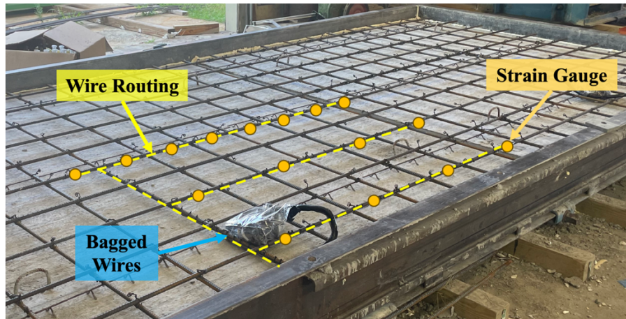
Figure 3.2-4: Typical strain gauge arrangement and protection
