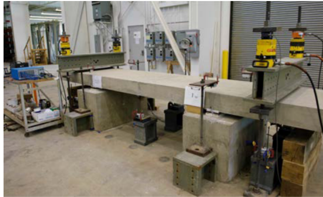
Figure 2.2-1: Constant moment test for slab specimens by Frosch et al. (2014)
