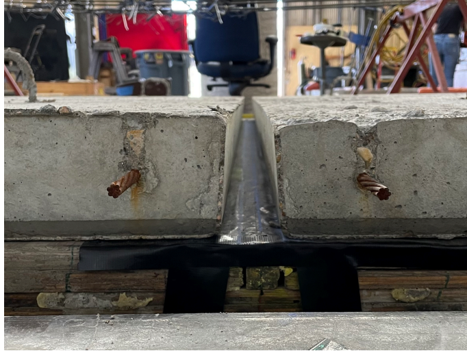
Figure 3.2-6: Longitudinal specimen panel joint details
