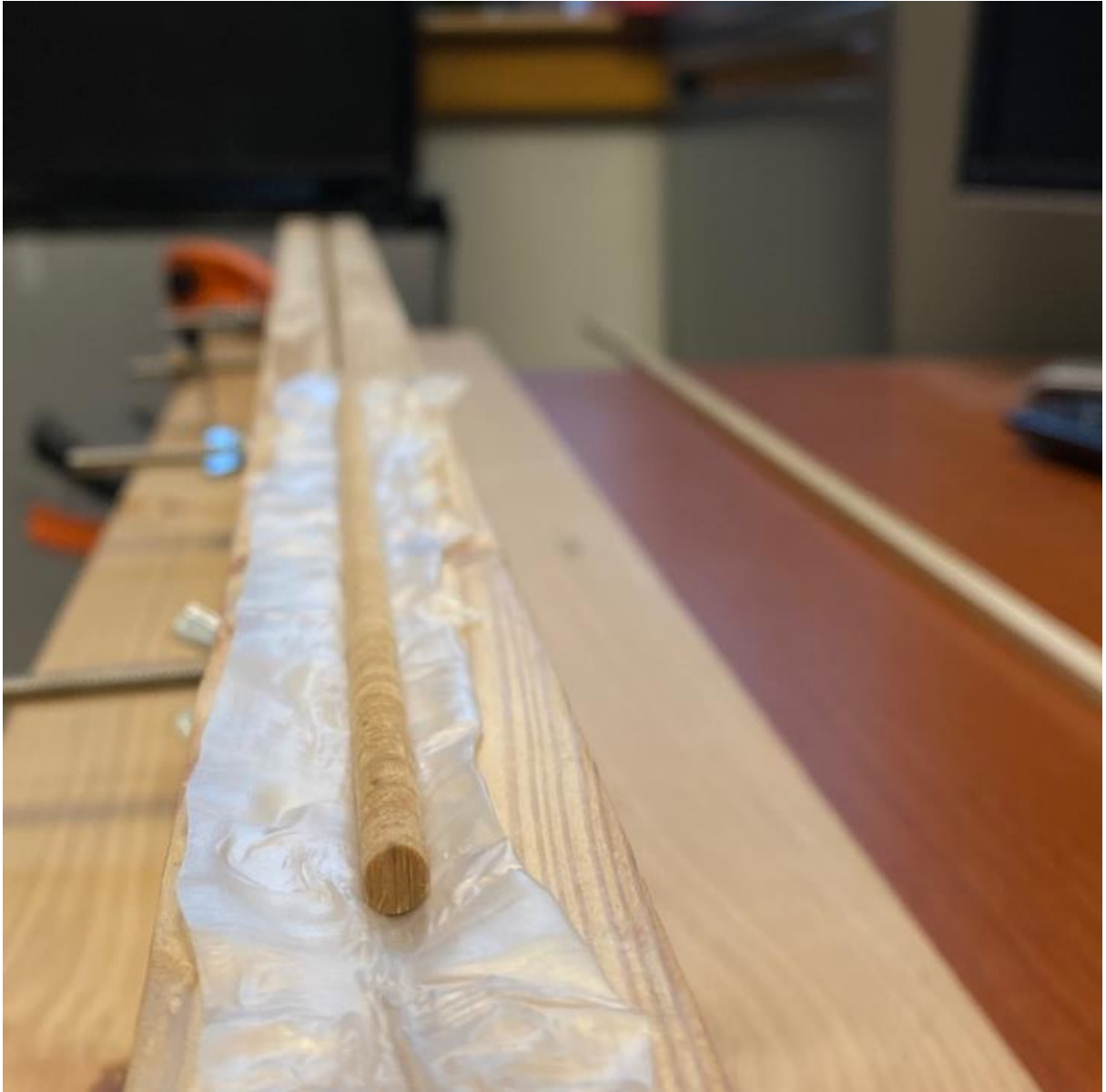
Supp. Figure 1: New core preparation method. The wooden vise-like device created for this study and used to hold tree cores in place without adhesive while a flat surface is planed with a stainless steel razor blade.
