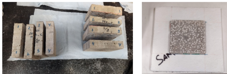
Figure 3. Sample preparation for thermal conductivity testing.
