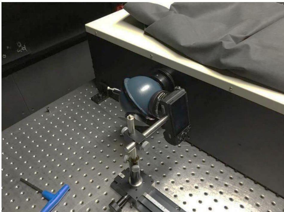
Figure 4.4. Camera positioned with its lens covering the opening of the integrating sphere. A black cloth was used to cover the camera and sphere to block any light from external sources contaminating images.
