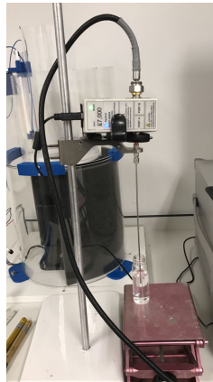
Fig. 3.2 Dielectric material measurement setup using probe kit and VNA.
