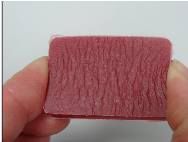
Fig. 6.21: Surface creasing of Parylene coated test sample.
