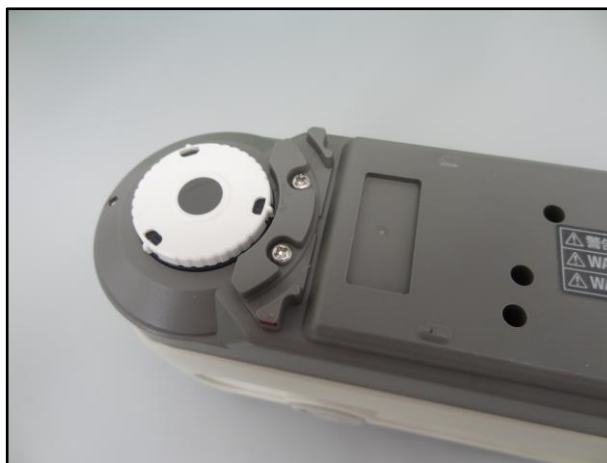
Fig. 3.5: Measuring head aperture of the spectrophotometer.
