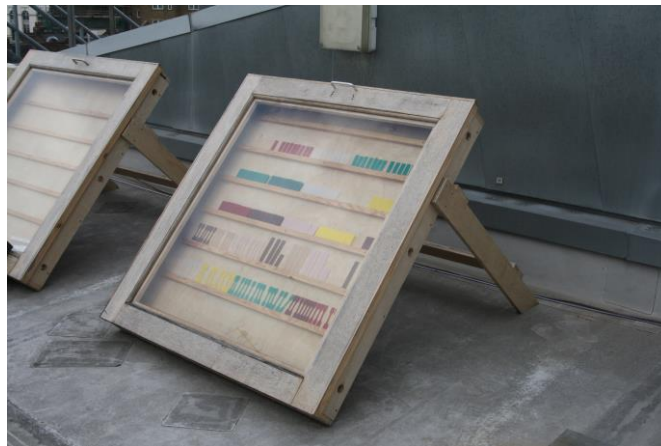
Fig. 3.4: Natural outdoor weathering of test specimens.
