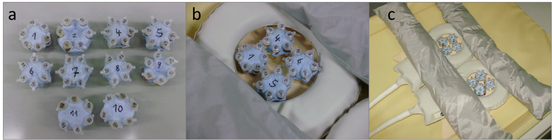
Figure 89: First MRI phantom. 0.5 ml Eppendorf tubes arranged around blu-tec putty. a: Several phantoms, one for each SPION. b: Four phantoms in a flex receiver coil. c: Eight phantoms in two flex receiver coils.
