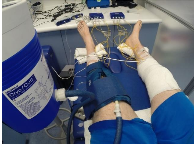
Figure 63 Supine position set with Cryocuff and RJB over respective knees on top of the pressure pads, with tubing connected to the Pasco quad pressure sensors and the Sparklink connecting them to the software on the laptop
