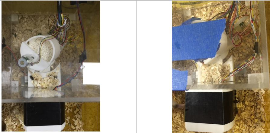
Figure 7.13 - Top view of a drop sensor jam due to cage bedding.
