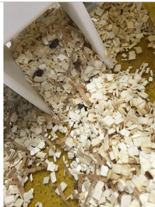
Figure 7.14 - Slit sensor and slit jam due to cage bedding.
