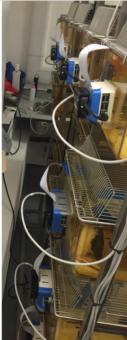
Figure 8.3 - Rear view of a typical cage rack with RatBot infrastructure.
