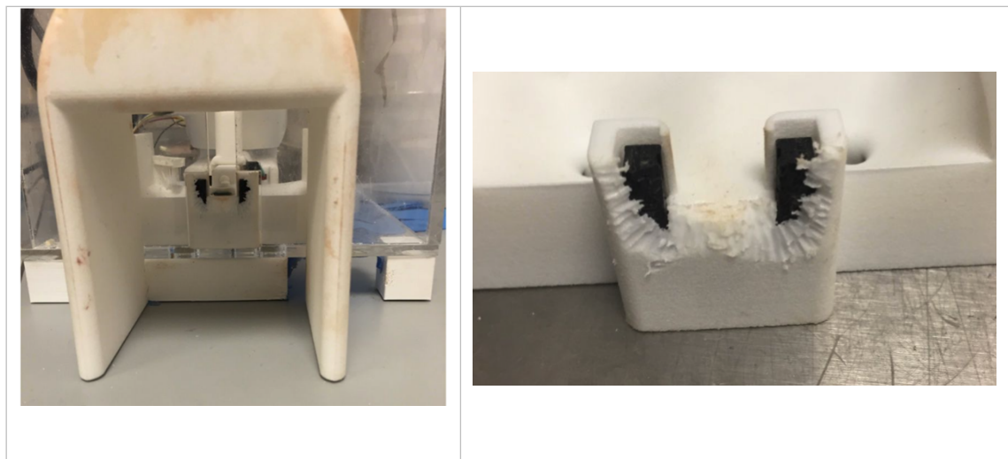
Figure 8.16 - Slit sensor bitten through during normal device operation.
