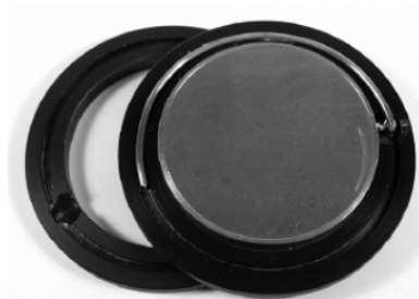
FIGURE 2.4: Circumference antenna on a pacemaker [9].
