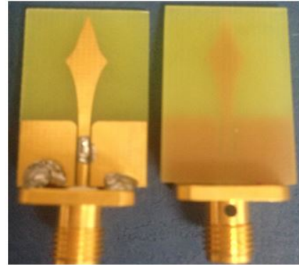
(b) UWB antenna Operating frequency 3.3 GHz – 6.2 GHz
