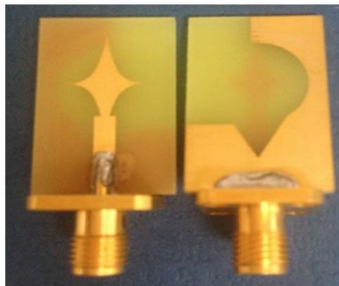
(c) UWB antenna Operating frequency 2.7 GHz – 10.9 GHz
