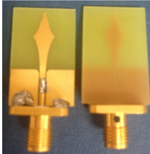
FIGURE 4.4: Prototype of CPW UWB Antenna (left) top view, and (right) bottom view.
