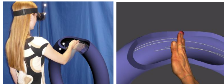
Figure 4-16 Hand-displacement-based pseudo-haptics (HEMP) (left) and the view the users see (right) [182]
