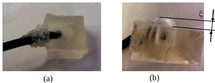
Figure 5-12 (a): Non-activated pneumatic haptic feedback actuator; (b): activated pneumatic haptic feedback actuator without the top silicone layer.
