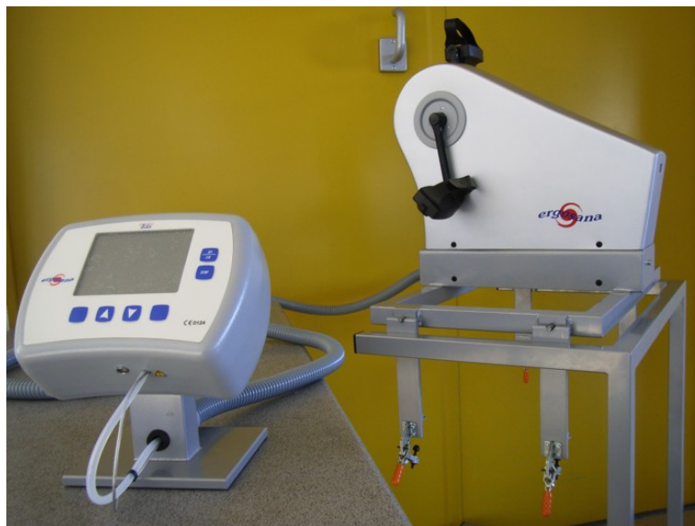
Figure 22. Supine cycle ergometer (Ergosana®, Germany) with purpose made mechanism to and from, and to attach to, the catheter lab table.
