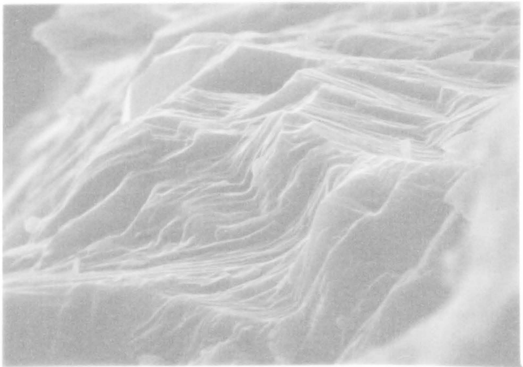
Plate 3.2. Electron micrograph showing lamellar structure of PEG 4000 in 7% w /w trimethoprim dispersion
