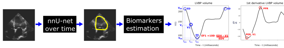
Fig. 1. Overview of the proposed framework to segment the left ventricle blood pool (LVBP) from echocardiography apical 4Ch images and to derive the systolic and diastolic clinical biomarkers.
