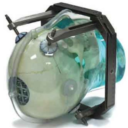
Inter-cranial Grid Phantom 335 Physical Control Points
