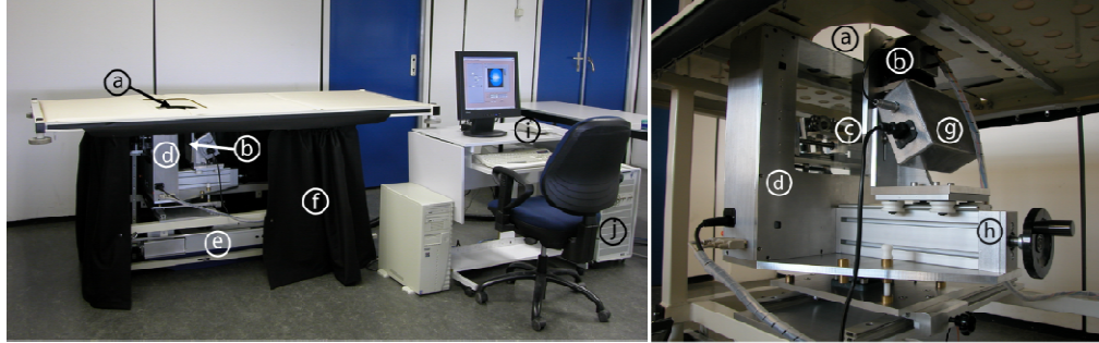
Fig. 1. The Twente photoacoustic mammoscope. a) Aperture to insert breast. b) Ultrasound detector matrix. c) Glass window. d) Scanning system compartment. e) Q-switched Nd-YAG laser operated at 1064 nm with 10 ns pulses. f) Laser safety curtain which is drawn around the instrument during the measurements. g) Interface electronics between detector and computer. h) Linear stage carrying detector matrix driven by hand wheel to apply mild compression to the breast. i) Laser remote control unit. j) Laser power supply. Image adapted from reference [27] with permission.
