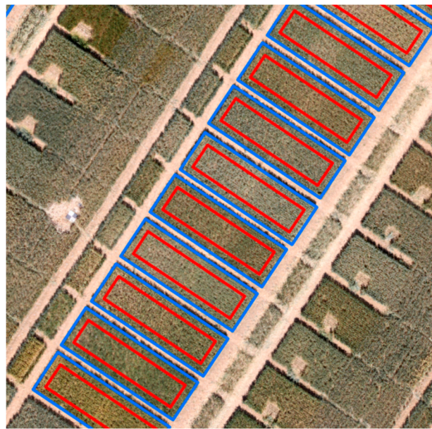
Figure 6. Plot borders before (blue) and after (red) buffering isolating each plot within the field in order to extract heights.
