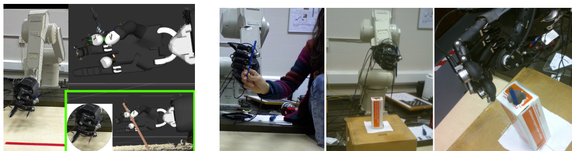
(a) Clockwise from left: Robot grasping the pencil; Point cloud overlaid with the robot model; Result of the pose estimation
