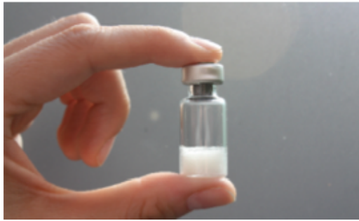
Glass vial containing the ARSOLux biosensor
