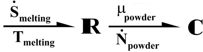
Figure 6.6: Proposed Bond Graph Modification: Additional Multi-port R Element
