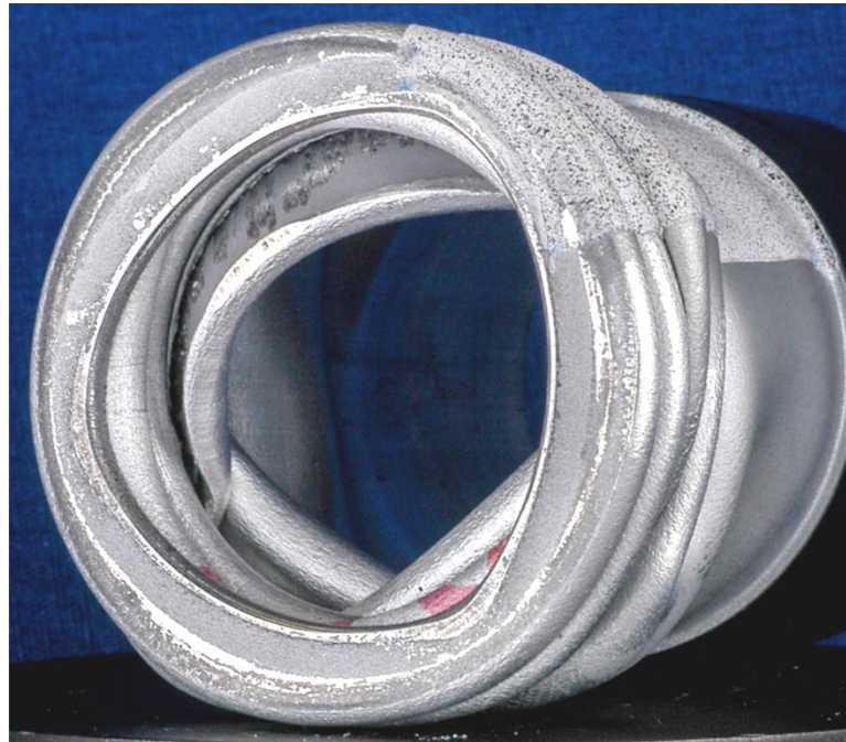
Fig. 2.13: Images of the specimen CR16 crushed. (a) Side view and (b) top view.
