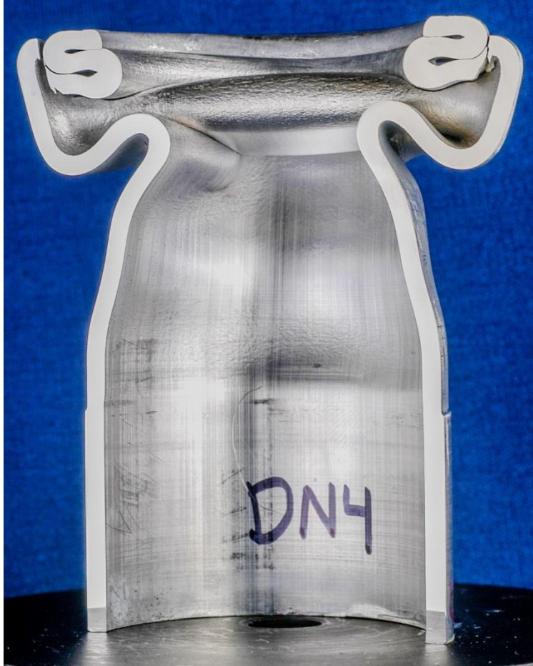
Fig. 2.17: Photograph of specimen cross section from experiment DN4 showing the protrusions that has torn through the thickness.
