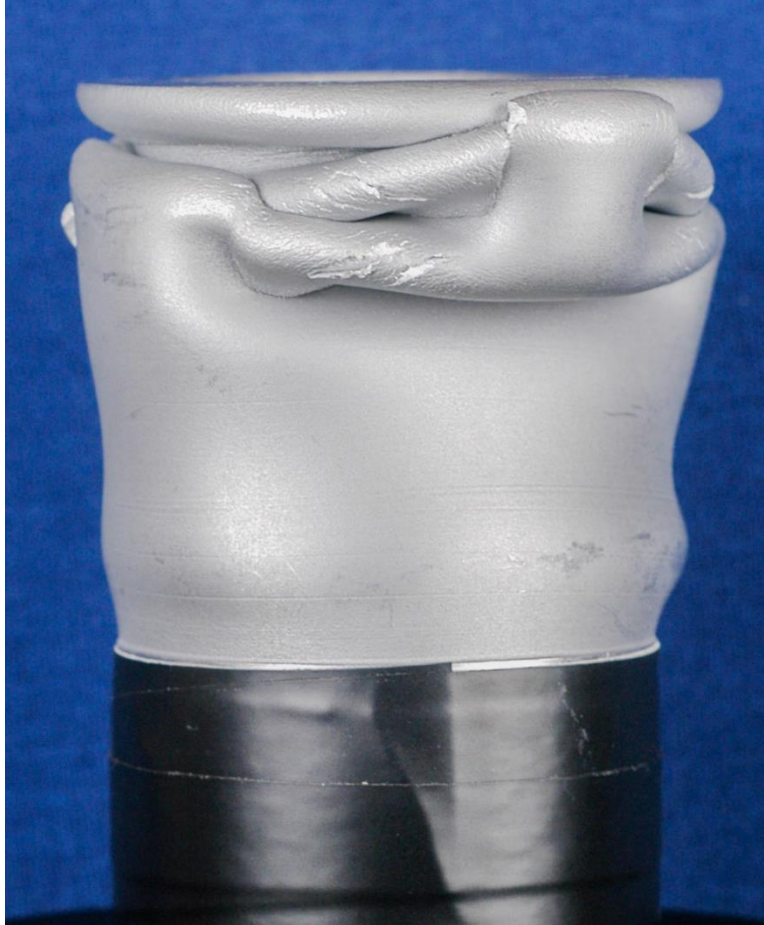
Fig. 2.16: Image of the specimen DN4 crushed showing failure during mode switch.
