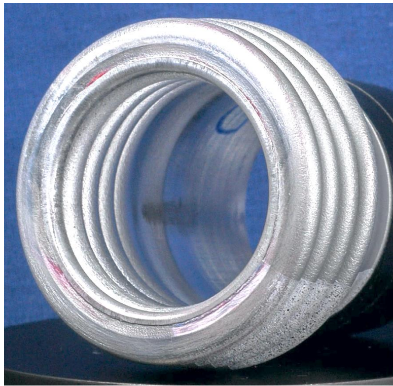
Fig. 2.11: Images of the specimen CR14 crushed. (a) Side view and (b) top view.
