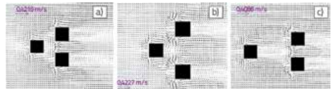
Figure 11. Average velocity vectors around piles (Case of 1x2 arrangements) away from bed by 0.01 of water depth for F_t = 0.50
