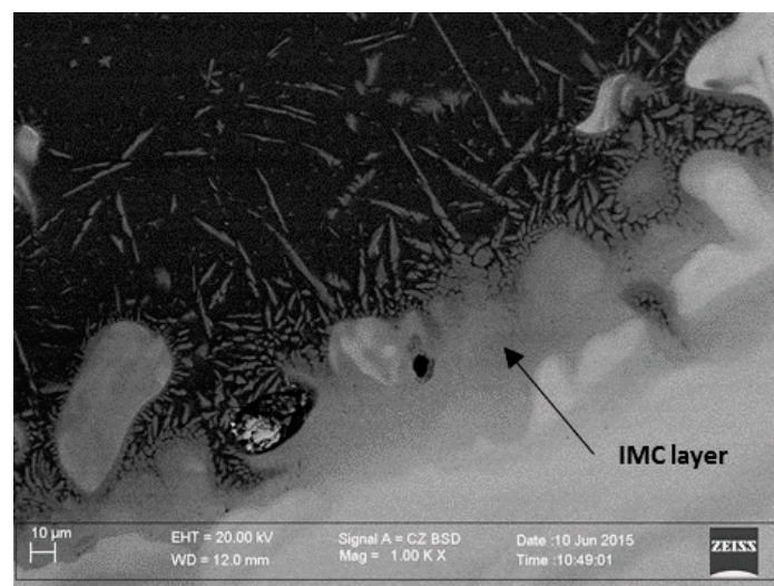
Figure 9. SEM Micrograph of intermetallic compounds (IMC) layer at the Al/Ti joint interface.
