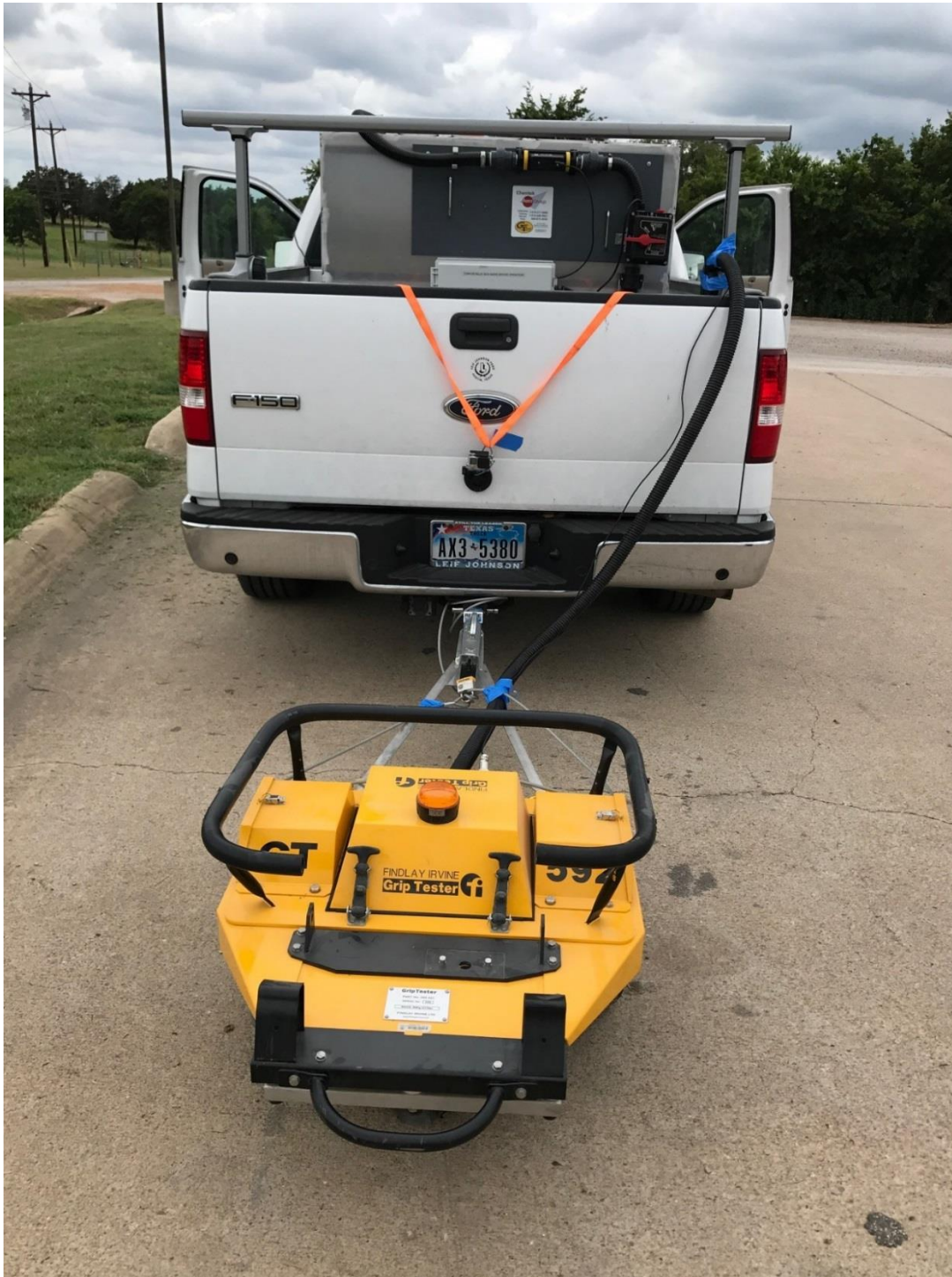
Figure 4.3: The Grip-Tester attached to a vehicle.
