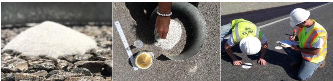
Figure 2.4: Sand Patch test.
