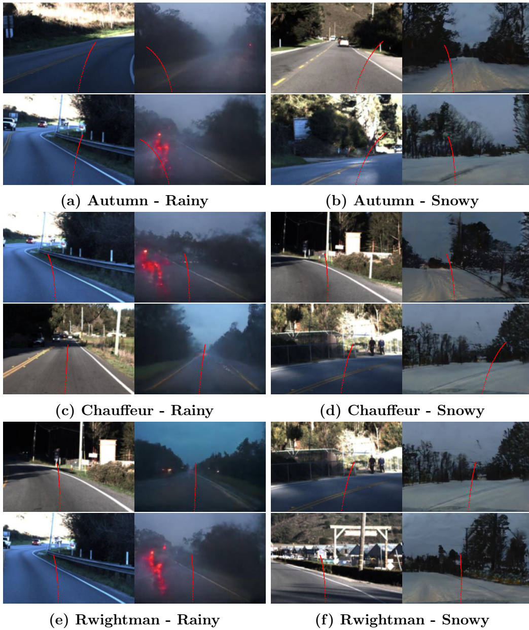
Figure 3.10: Inconsistency of Steering Angle Prediction on Original and Synthetic Images
