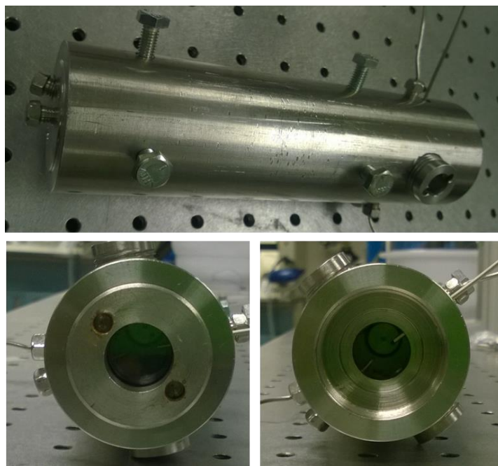
Figure C.3. Images of the high-pressure methane hydrate cell.
