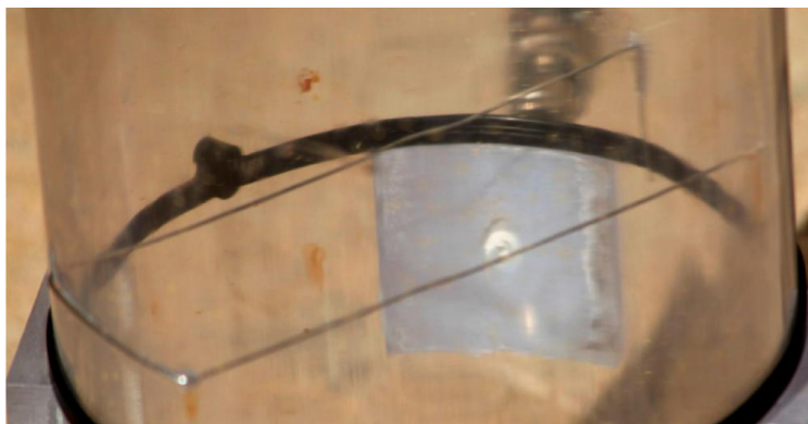
Figure 4-4: Packing support used in single phase dry pressure drop studies. Figure taken from Owens. 62
