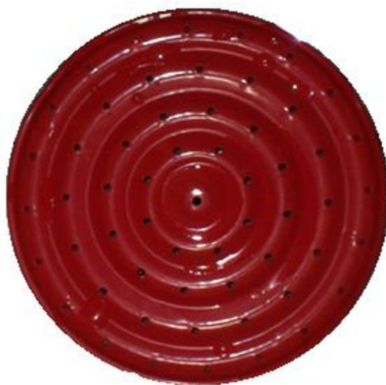
Figure 4-3: Top view of the vapor distributor used in dry pressure drop studies.
