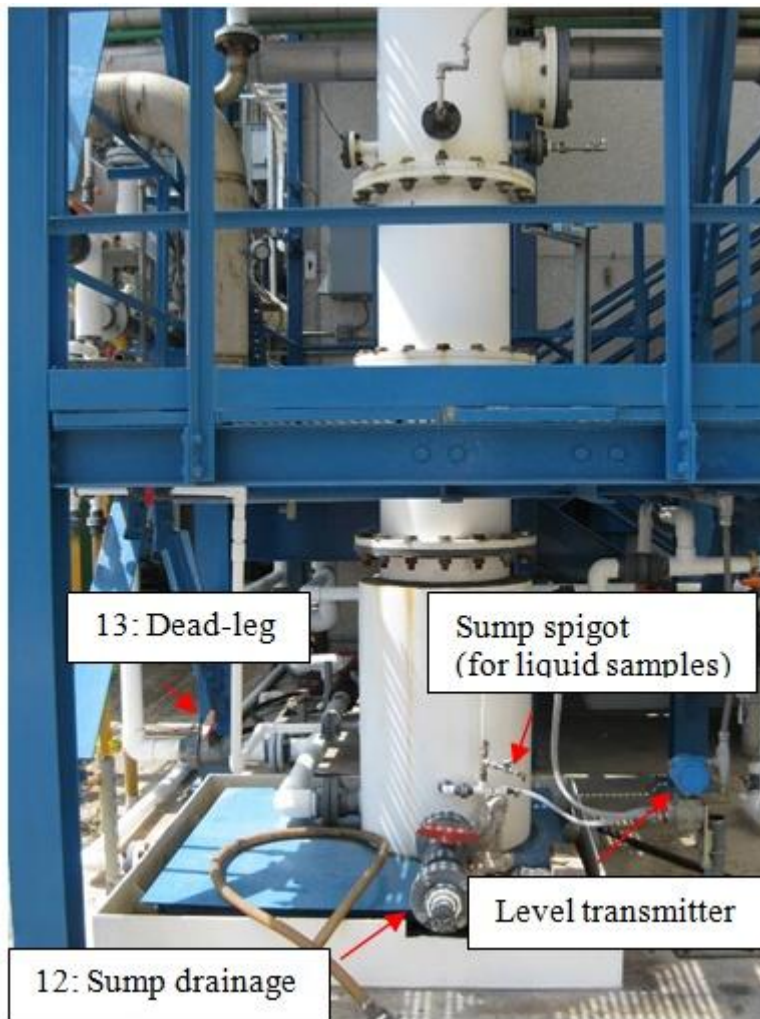
Figure B-6: Column sump.
