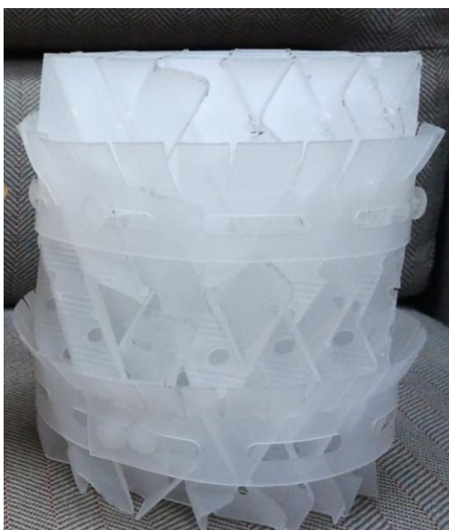
Figure 4-1: Sample half element of Mellapak N250.Y used in experimental work.
